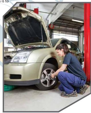
\* Finish tightening the nut to the correct torque. Ensure that the torque wrench is squarely on the nut and the nut is in good condition. Any slippage will create an incorrect result.
